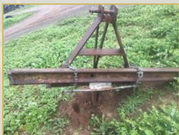
Ripper with spray nozzles.
