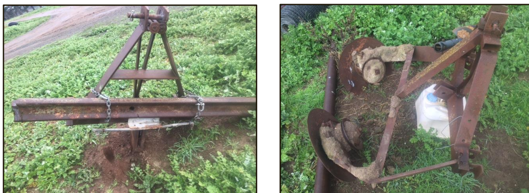
Figure 12. Homemade ripper with sprayer attached (left) and two-disk moulder (right) used in some Landcare planting projects.
